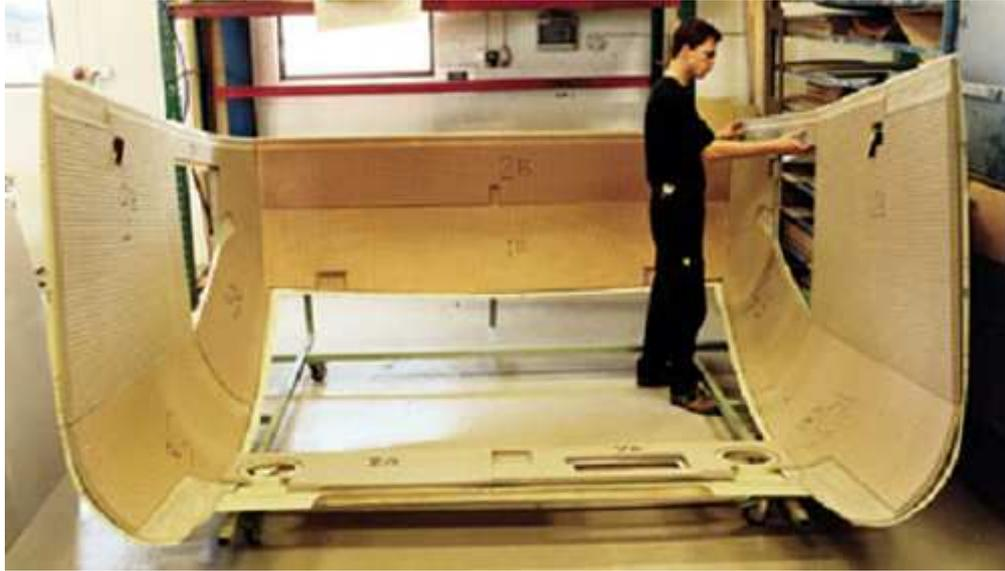
Figure 13: Laying up a composite train with Divinycell Cores (Railway Technology, 2012)
