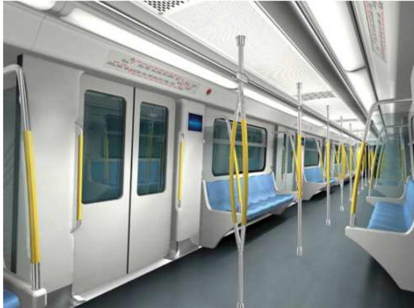
Figure 15: KTK Group interior components utilise DIAB core materials on the new Shanghai metro (McConnell, 2008).
